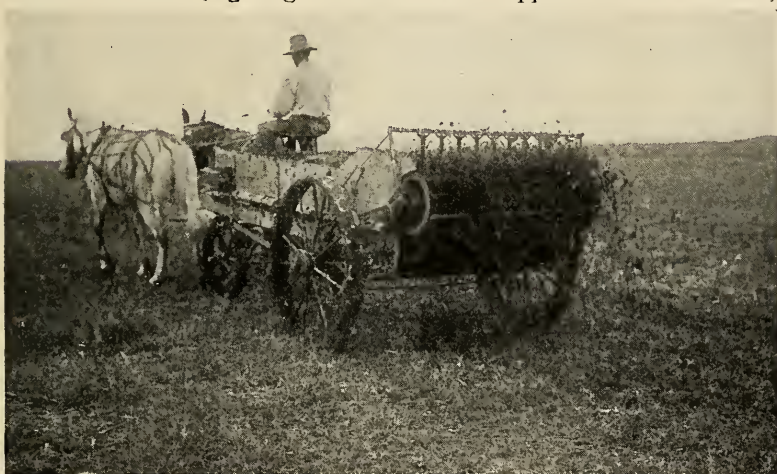
FIG. 83.—Manure spreader in action. The manure is torn apart so as to be scattered uniformly. (J. C. Beavers, Cir. 49 Purdue Station.)
